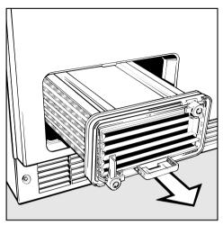
Pull out the heat exchanger.
